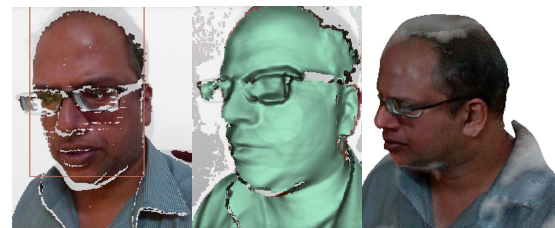
Fig. 8. Image of an object with transparent surface (spectacles) captured and reconstructed using BSMV RGB-D method.
